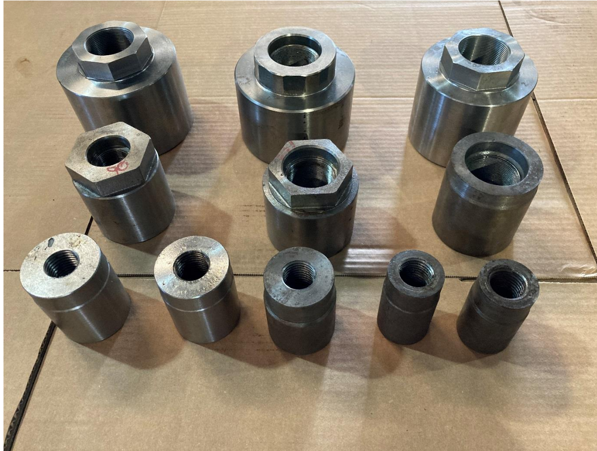
Plunger tips manufactured on gray iron
